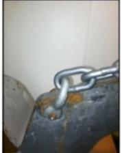
Slip Anchor Saver Shackle through the shank eye hole. Use Stainless Steel wire tie provided to slip around the anchor shackle arm. This prevents you from losing your shackle after a break a way). (Do not over tighten wire tie.)
